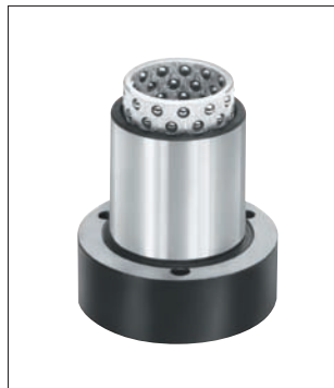
Long version Cage travel = 1/2 length of stroke
