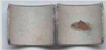
Fig. 35: Local damage caused by cavitation
