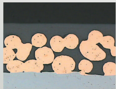
Fig. 4: Condition of sliding surface in the initial state
