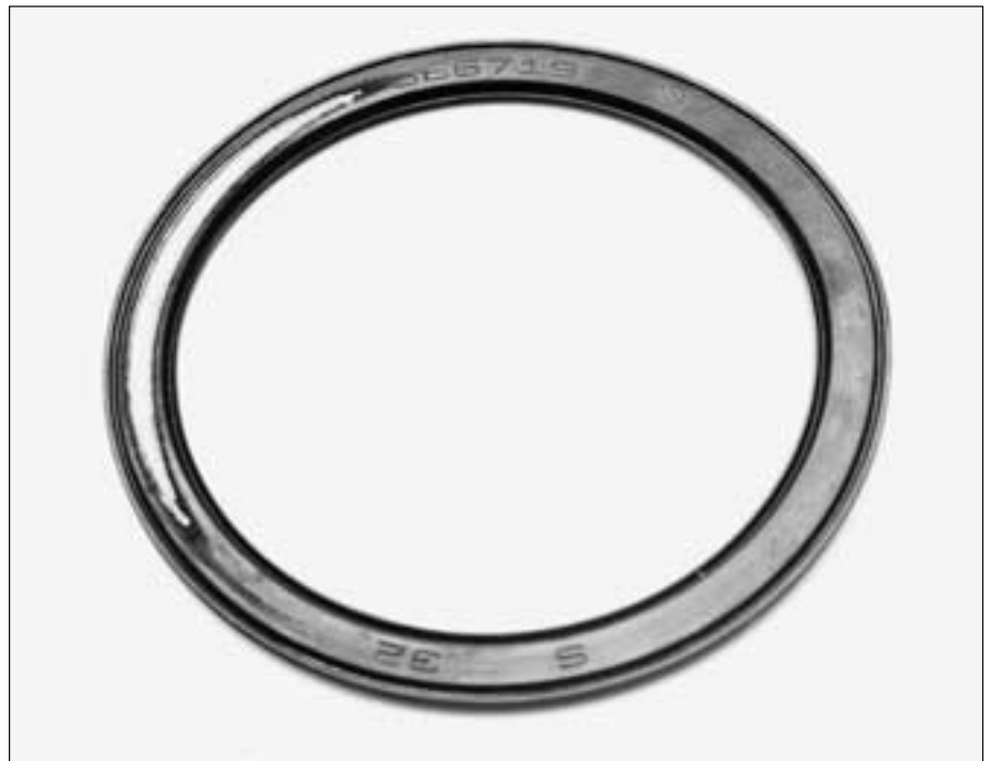
22: Seal damage due to lateral grazing
