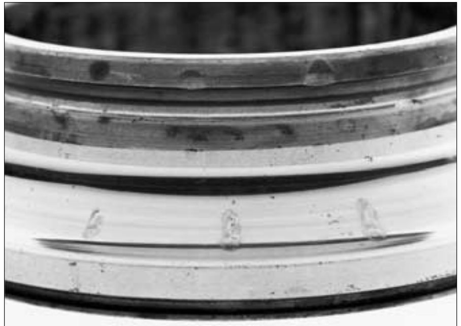
57: False brinelling on the ball bearing
