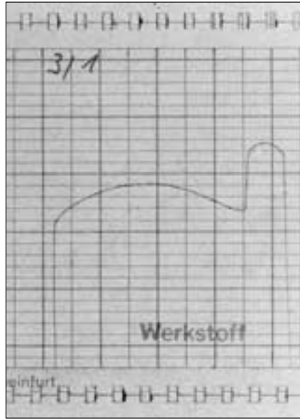
83: Cross profile chart of a worn tapered roller face
