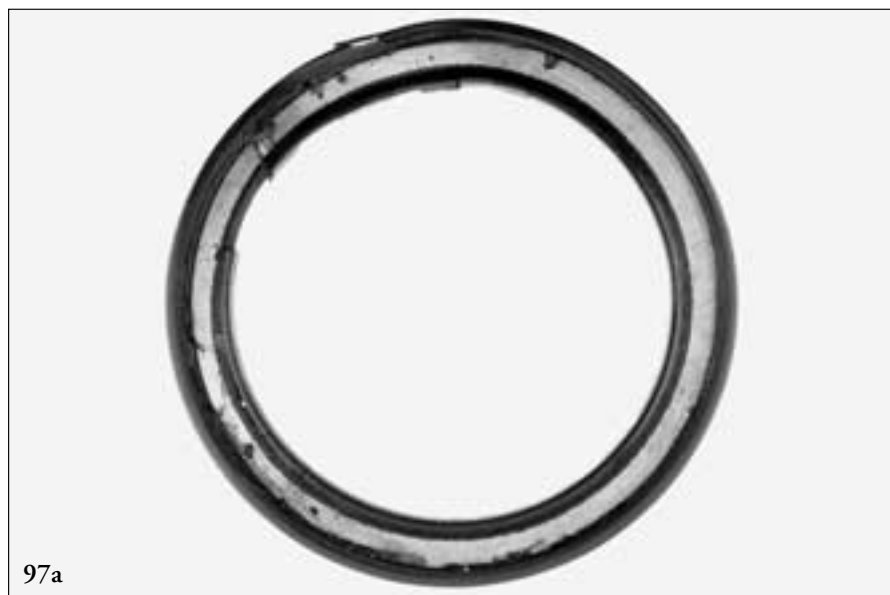
97: a: Hardened sealing with wear and fractures
