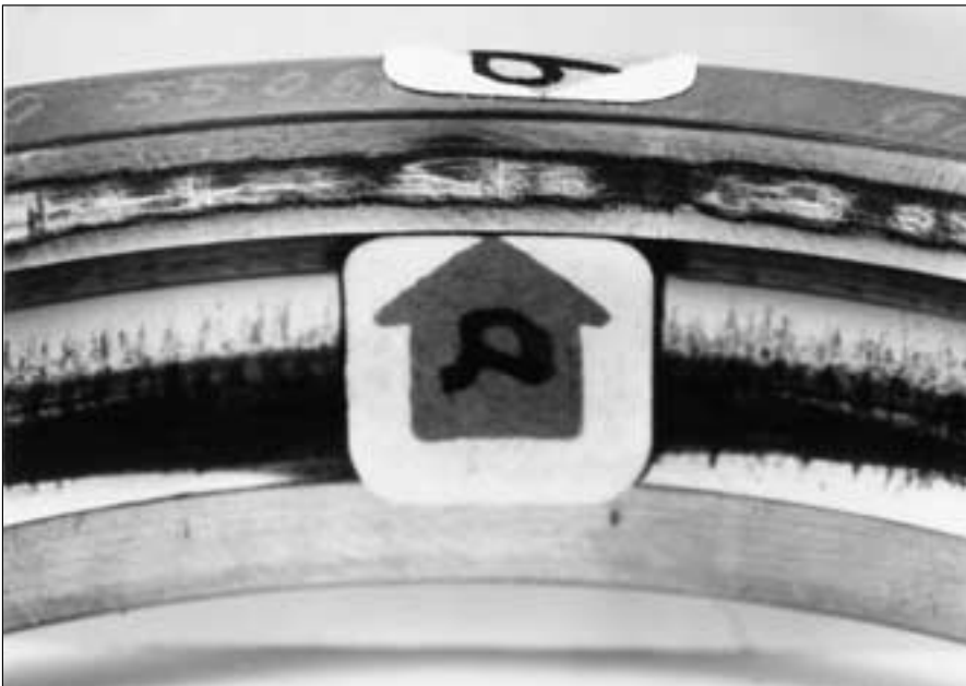
86: Bad contact marks on the cage guiding surface of an outer ring lip with smeared on material
