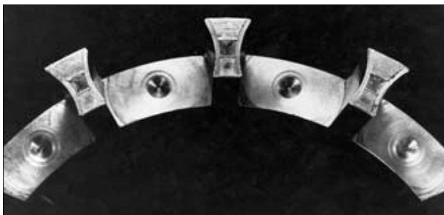
92: Fractured cage-rivet connections may result from vibration stress.
