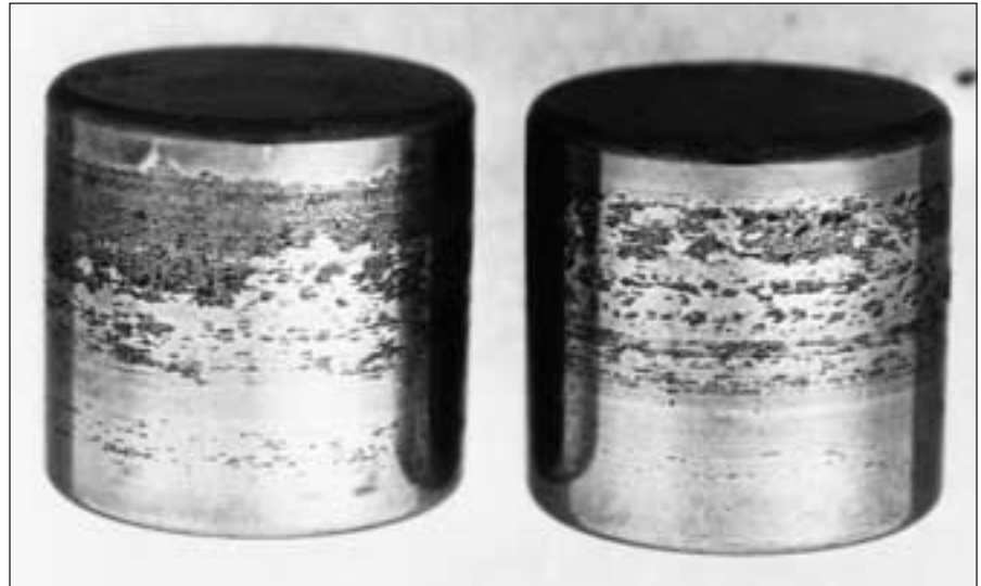
74: Slippage tracks on cylindrical rollers
