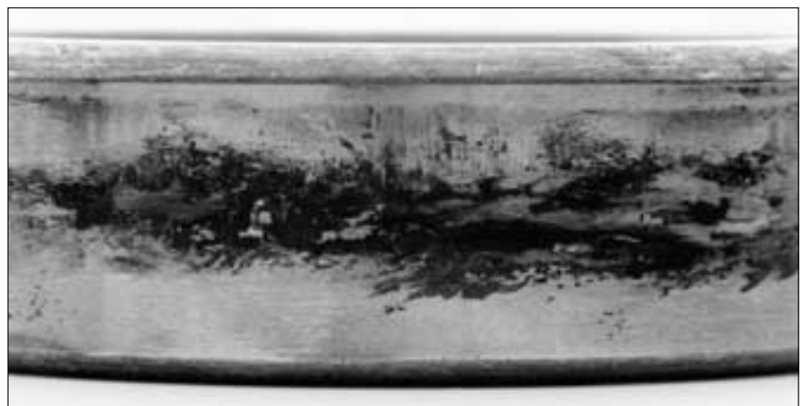
14: Fretting corrosion reveals the size of the load zone at the stationary outer ring
