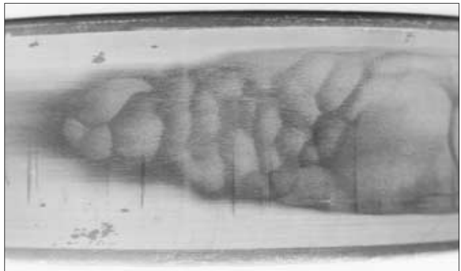
75: Slippage damage on the inner ring of a cylindrical roller bearing
