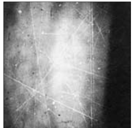
48: Fatigue at the raceway edge in the case of ball bearings, e.g. with high moment load (edge running); left raceway edge, right ball.
