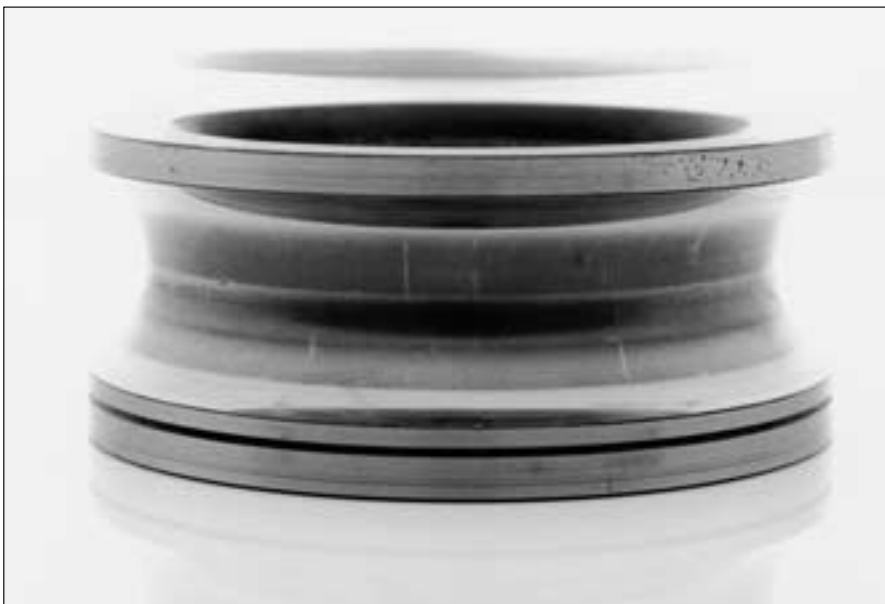
28: Track with surface wear
