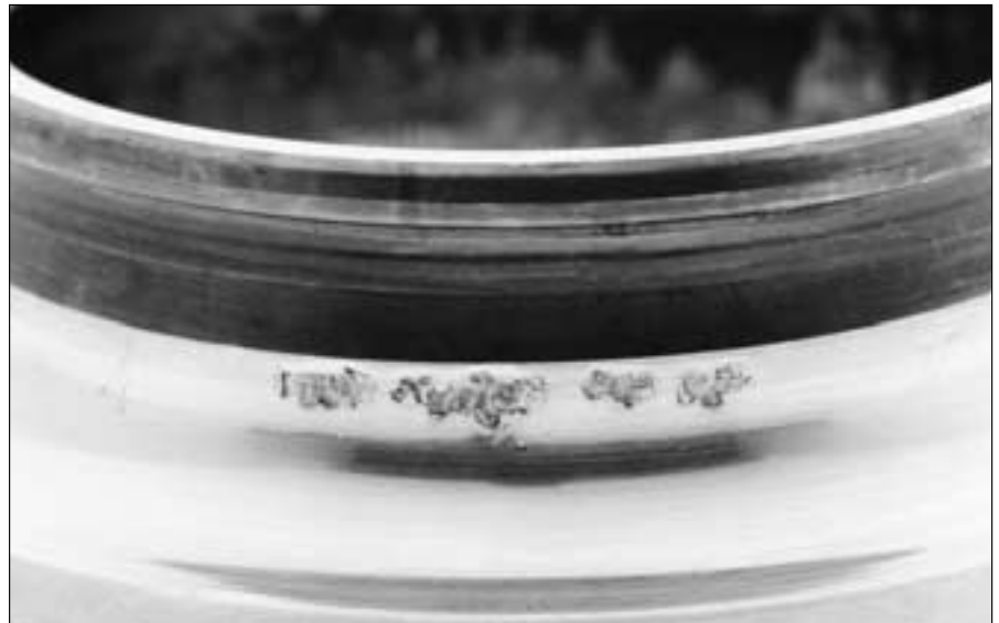
46: Fatigue damage in groove bottom of an angular contact ball bearing's inner ring as a result of insufficient adjustment force
