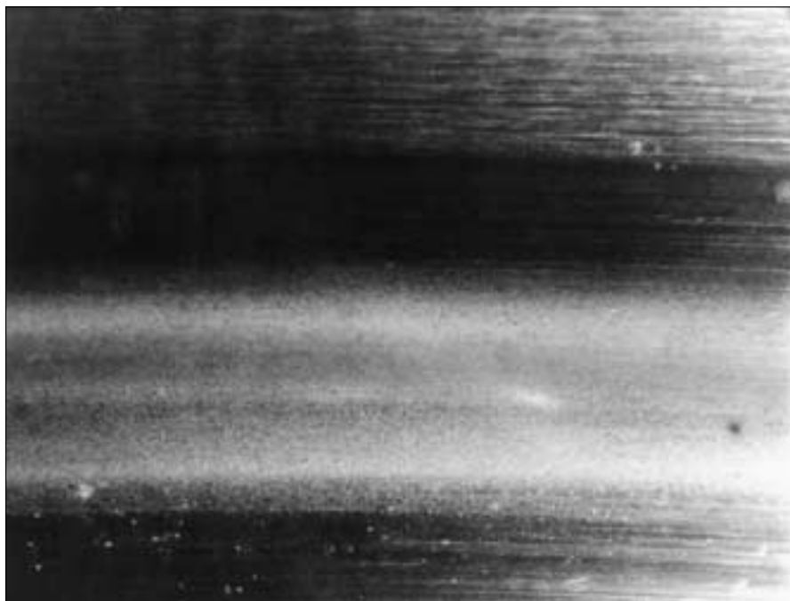
66: Worn, roughened raceway
