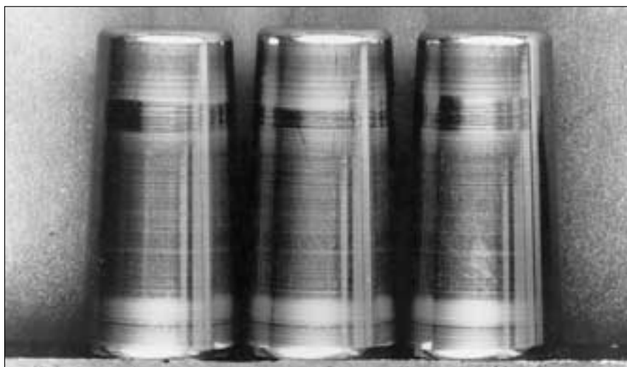
67: Wear traces can usually first be detected on the surfaces of the rolling elements
