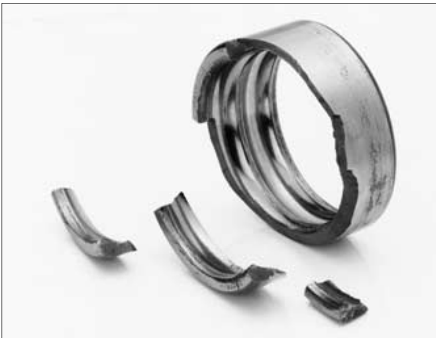
65: Crack in outer ring in circumferential direction
