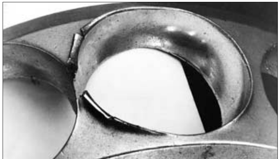
91: Bearing rings tilting towards one another led to high constraining forces between balls and cage which, in turn, led to web fracture.
