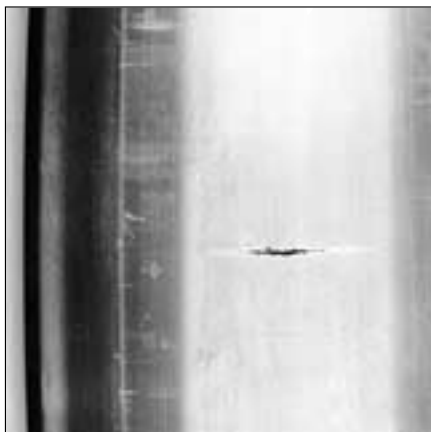
6: Inner ring damage to a spherical roller bearing in a paper making machine found by means of the envelope detection procedure.
