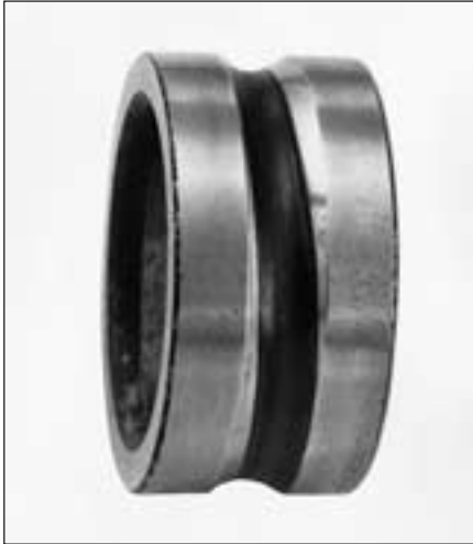
39: Oblique track in inner ring of deep groove ball bearing
