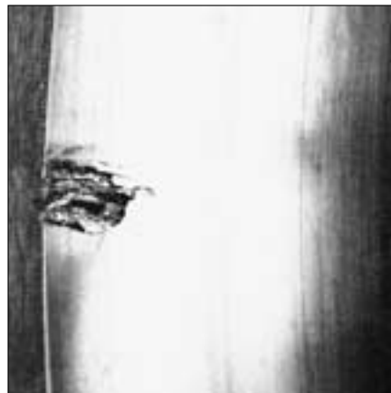
48: Fatigue at the raceway edge in the case of ball bearings, e.g. with high moment load (edge running); left raceway edge, right ball.
