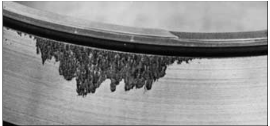
48: Fatigue at the raceway edge in the case of ball bearings, e.g. with high moment load (edge running); left raceway edge, right ball.
