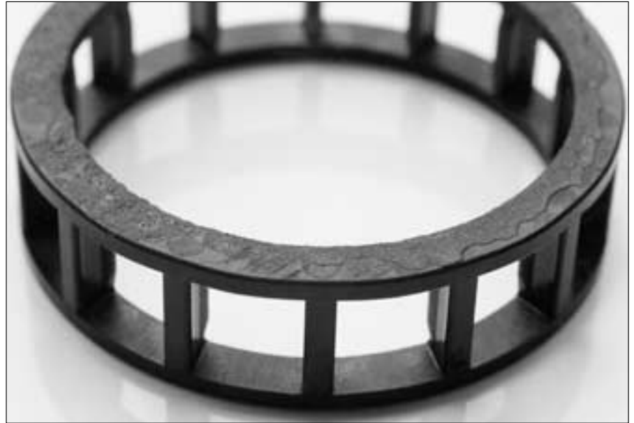
94: Melted faze of plastic cage in the case of incorrect bearing heating on a heating plate
