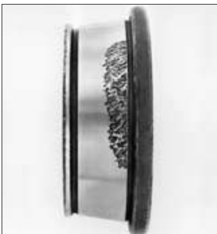
40: Tilted track on a tapered roller bearing
