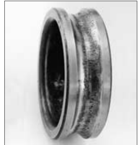
42: Advanced fatigue damage on deep groove ball bearing
