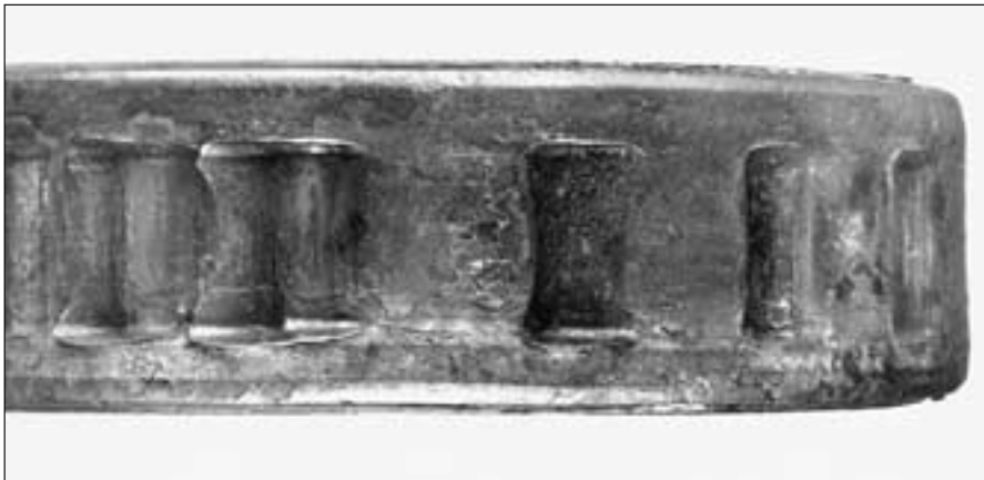
77: The rollers left deep impressions in the raceway of a seized, overheated cylindrical roller bearing.
