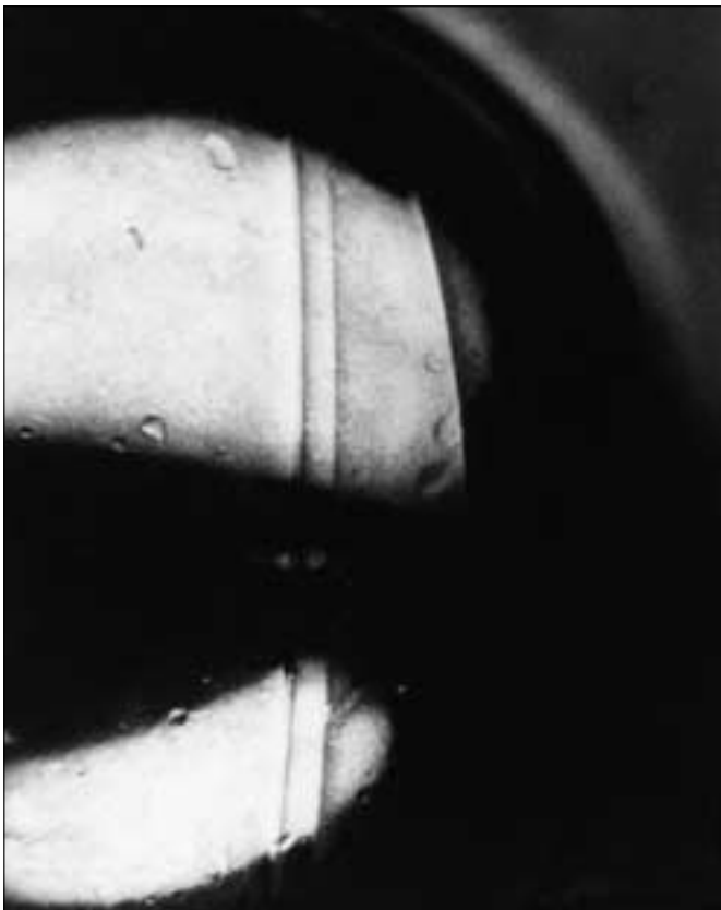
61: Ball with extreme edge tracks caused by long-term constant load
