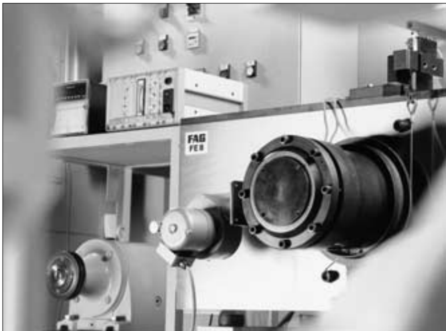
107: Test rig for determining lubricant quality
