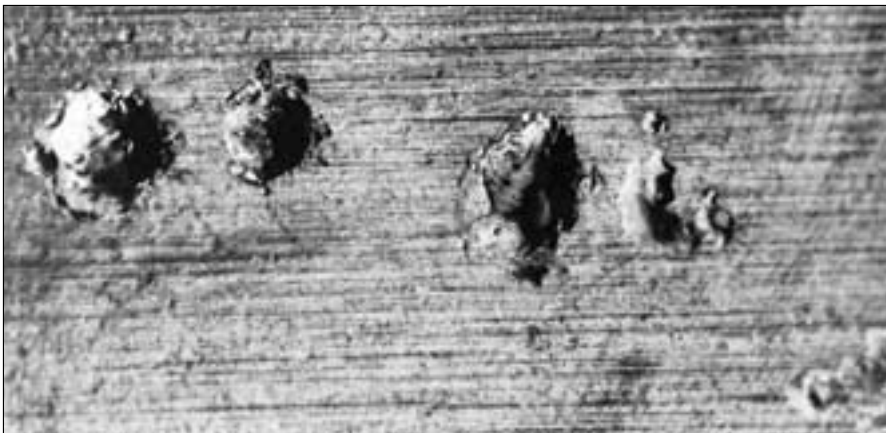
59: Current sparkover led to the formation of craters in the raceway of a cylindrical roller bearing.
