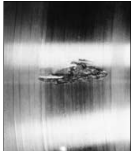
52: Failure mechanism as in fig. 51 but with wear of the raceway edges, cross profile of the roller see fig. 69.
