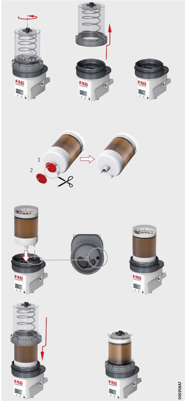
Figure 11 Fitting the lubricant cartridge
