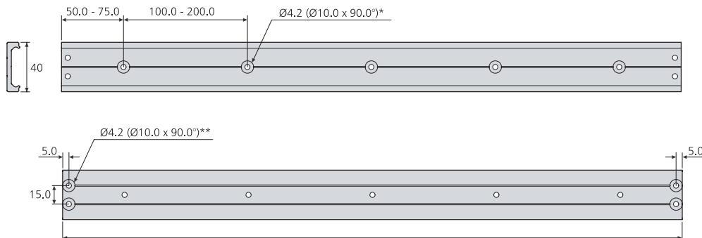
\* Fixing: drill 4.2mm holes on centre line, fully countersunk.
