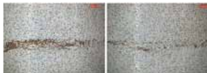
Fig. 35: Damage due to erosion in the running-in layer of a P1 plain bearing
