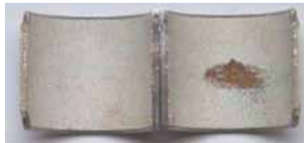
Fig. 34: Local damage caused by cavitation
